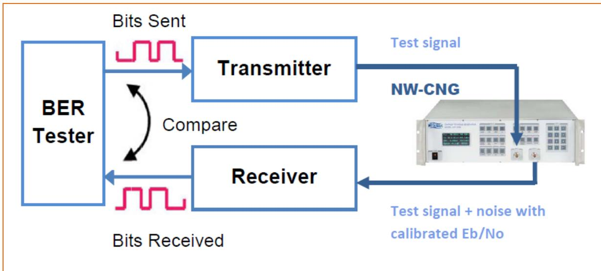
**Figure 2 Typical BER Test Application**
