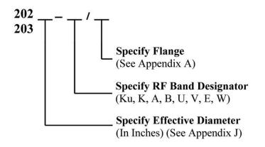
The center frequency should be specified when ordering these antennas. Beamwidths are typically  $\pm$  5%. Sidelobes are nominally -20dB. Boresight telescopes and boresighting are recommended and are available on request.
